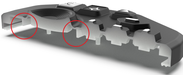
Image: Supporting walls around a key
