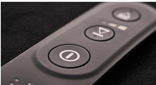
Image: Example of raised button area in a keypad
