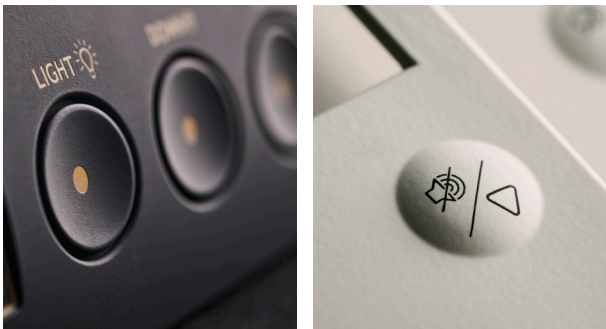
Image: Examples of concave and convex buttons
