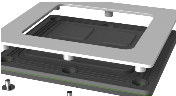
Image: Example of a sealing lip moulded as thin lines around the keypad edge
